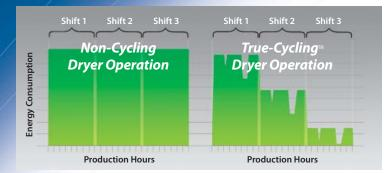
In applications with varying air usage and shift demands, and where there are daily and seasonal changes in ambient temperature, HeatSink™ True-Cycling™ operation provides a way for compressed air users to minimize energy cost associated with air treatment.
